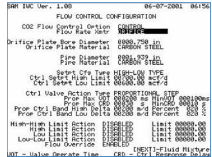
Orifice Plate and Control Configuration
